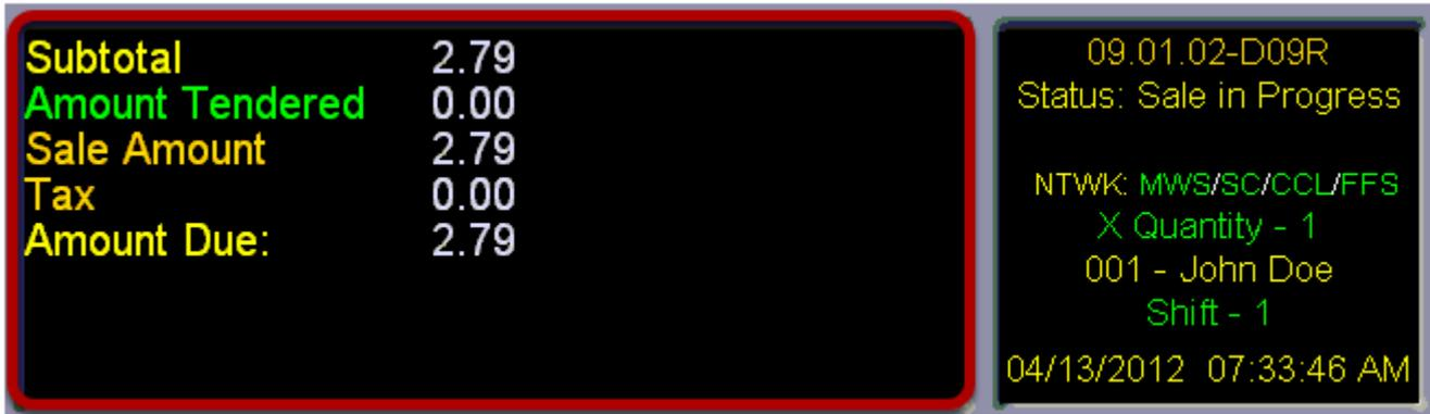
The **Main Display** is located in the top left portion of the screen and it used to display items in a sale, subtotals, and inquiries. When touched, the **Main Display** will toggle between your current screen and the fuel screen.
