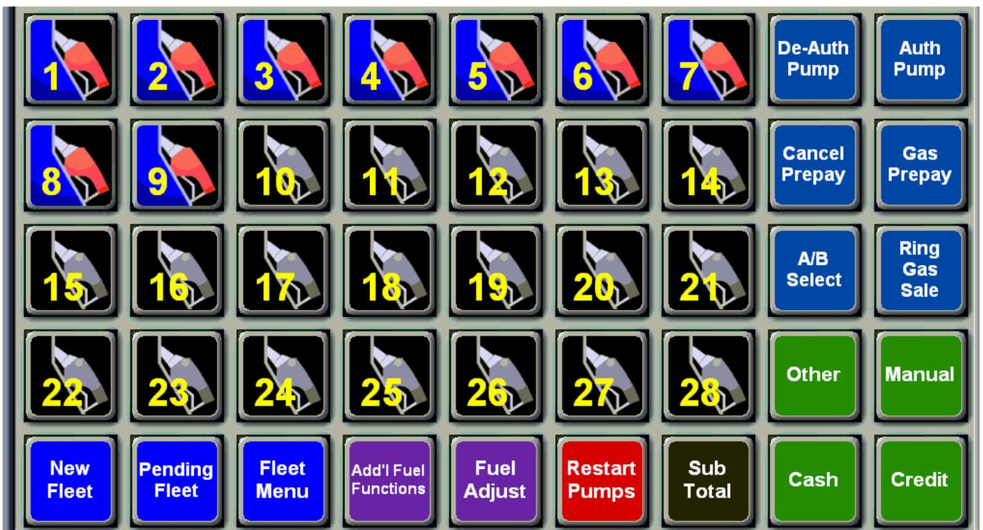
There are multiple banks of keys. These 2 examples are the home screen, which contains the most commonly used buttons and the fuel screen, which contains the dispenser icons and fuel related buttons.
